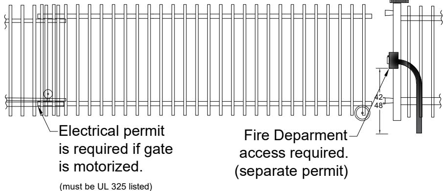
Fences and gates around pools must meet the requirements for pool enclosures (see pool enclosure standard). These drawings represent examples and are not intended for the purpose of design for a particular project. (additional Fire requirements may apply)
